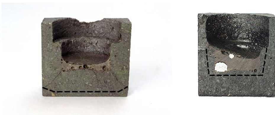
Figure 2. Cross sections of (a.) a conventional 90% chrome refractory, and (b.) ARC’s modified refractory following exposure to a coal slag at 1600° C. The depth of slag penetration is marked in each case.
