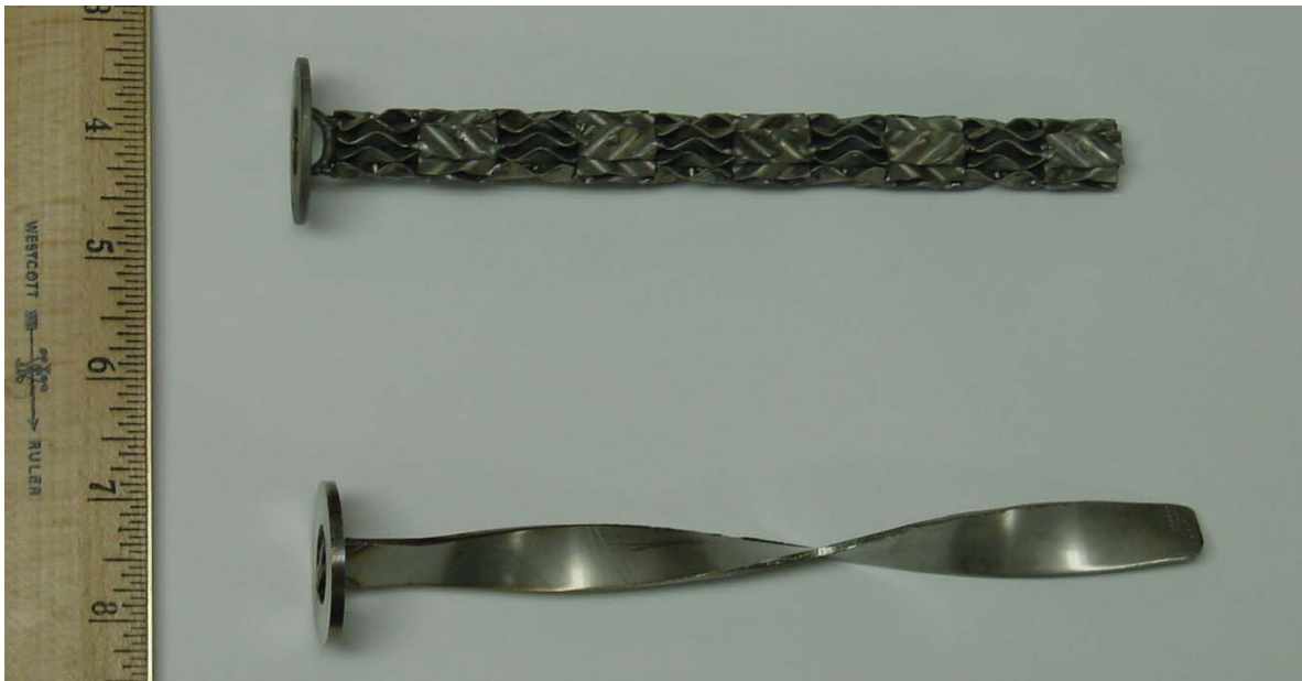
Figure 3 - Static mixers: high-mixing design (top) and spiral mixer (bottom).
