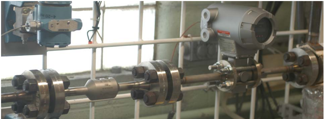
Figure 2 - V-cone flow tube (left) and electromagnetic flowmeter (right).
