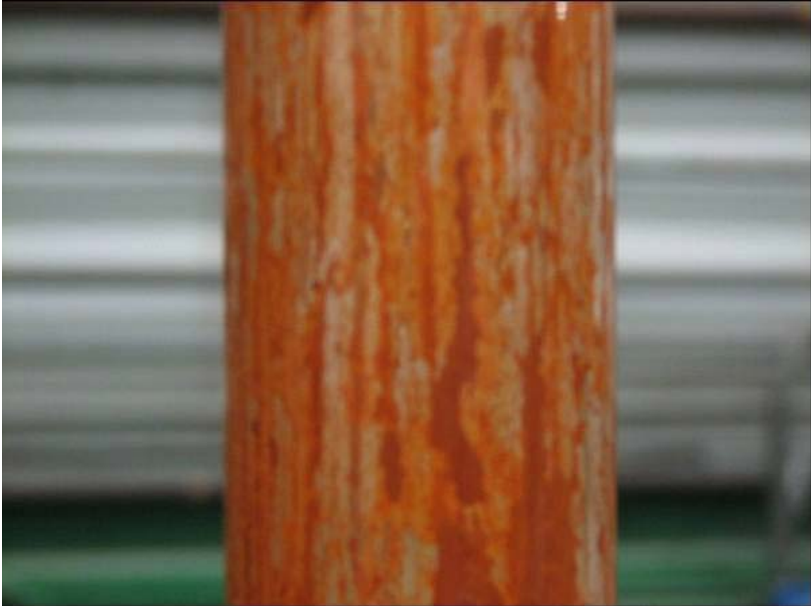
Figure 19. First Section after 400 Cycles of AZ-101, Test 15
