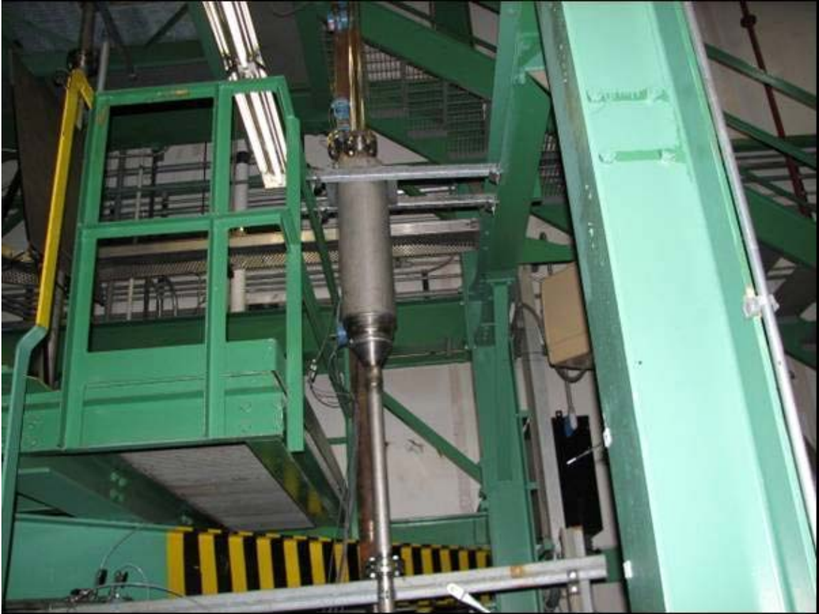
Figure 6. Photograph of Test Section showing 8" Dome used for Tests 14 & 15
