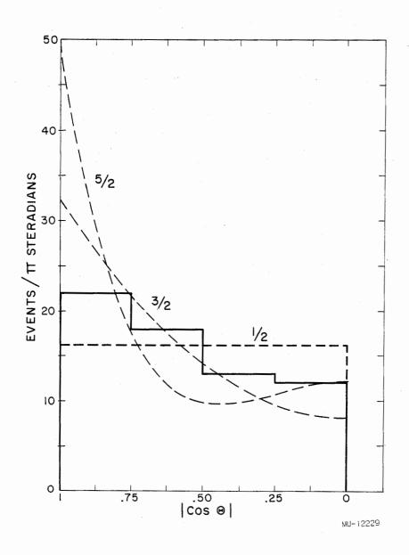
Fig. 6. Angular distribution of the pion produced in  $\Sigma$  decay. The histogram represents the sum of  $\Sigma^+$  and  $\Sigma^-$  events, folded through 90°. The three dashed curves represent the theoretical distributions for  $\Sigma$ 's of spin 1/2, 3/2, and 5/2 (the latter two are valid only if K<sup>-</sup> captured in a state of angular momentum 1/2). The thin solid line is the best fit to our data on the assumption that the distribution is of the form  $(1 + A \cos^2 \theta)$ .
