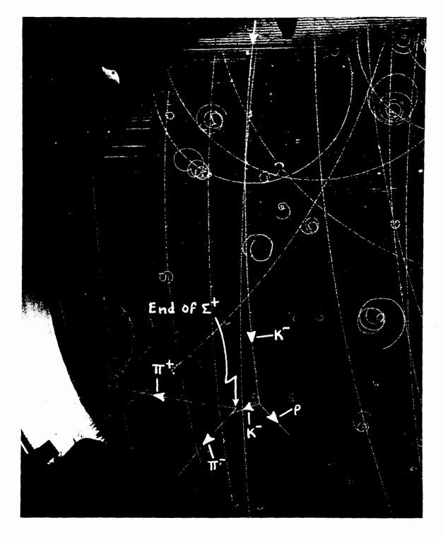
Fig. 2. A K<sup>-</sup> scatters elastically on a proton before coming to rest and forming a K-mesic atom. Then K<sup>-</sup> +  $p \rightarrow \pi^- + \Sigma^+$ ;  $\Sigma^+ \rightarrow \pi^+ + n$ . The horizontal lines spaced about 1 mm apart in the chamber are caused by light scattered in passing through a "Venetian blind" used in the dark-field illumination system.
