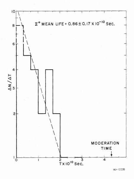
Fig. 5. Distribution in time of the  $\Sigma^+$  decays. Four short  $\Sigma^{i}s$  were found whose charge could not be determined. Two of these were arbitrarily called  $\Sigma^+$  and are represented by a dashed area.
