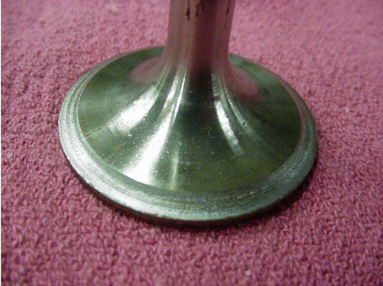
Figure 16. Excessive Valve Wear
