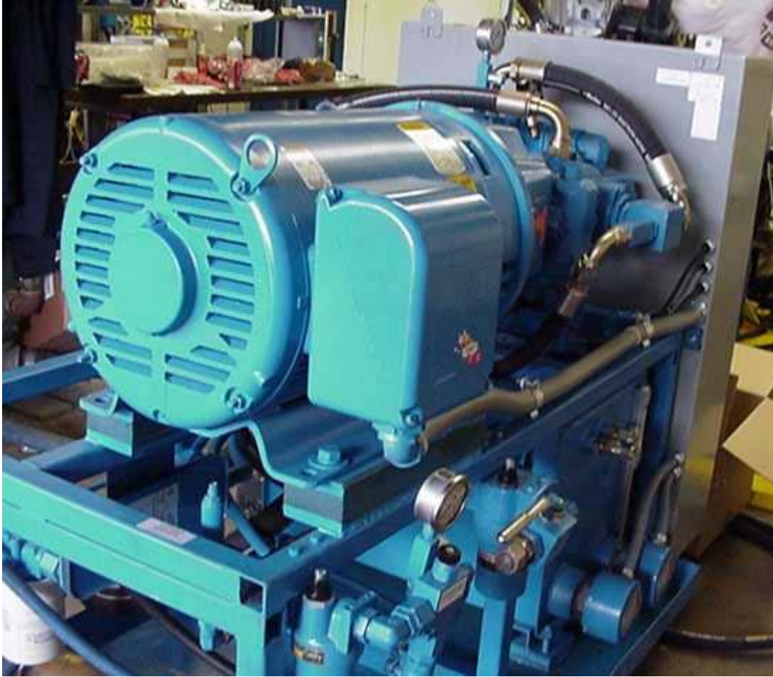
Figure 9. Hydraulic Pump Cart for the HVA System
