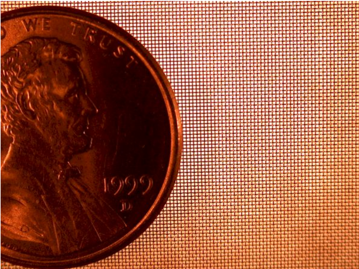
Fig. 2. Copper mesh 100x0.0045"
