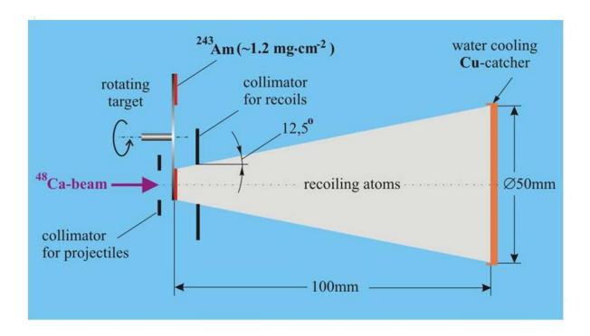
Figure 1. The target/Cu catcher block configuration for both the June 2004 and December 2005 chemical experiments.
