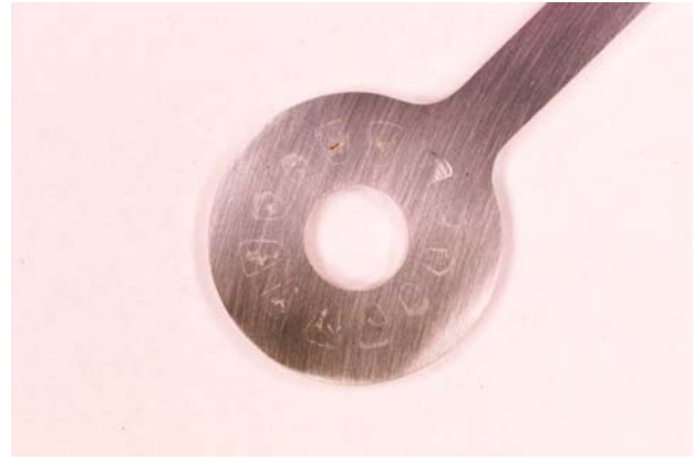
FIGURE 9 – Specimen JE1642 after CPP in BSW at 105°C. Scan Rate – 0.0167 mV/s. Small amount of crevice corrosion
