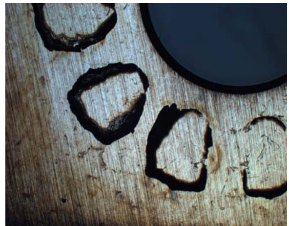
Figure 7. KE0691 after CPP test Crevice corrosion is observed
