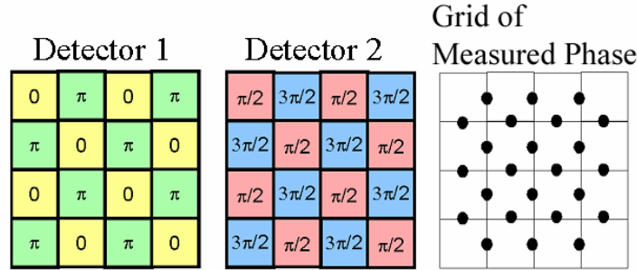
Figure 31: Pixellated phase shifts and wave-front measurement grid.
