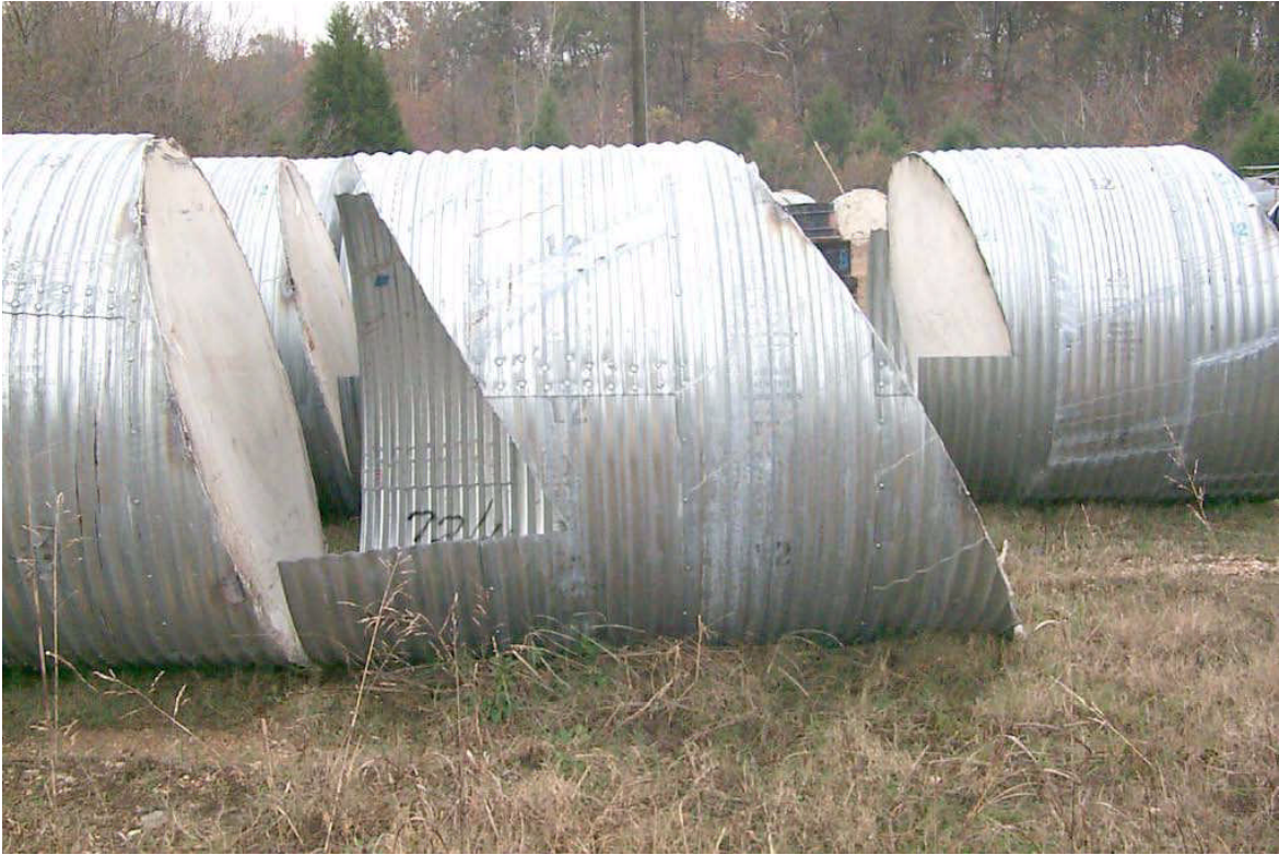
Figure 4 Target test sections showing cut face to produce impact angle.
