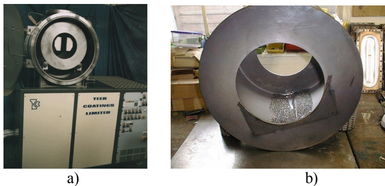
Figure 2- a) Picture of the barrel coating system b) Close-up picture of the barrel with some material inside (not our microspheres)
