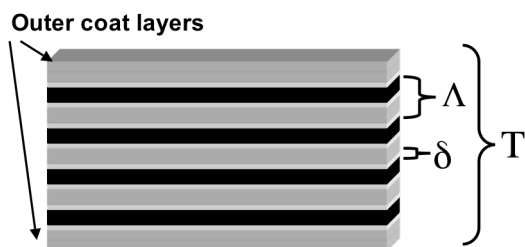
Scheme 1. The structural features of an energetic multilayer: The distance T is the total thickness of the multilayer, \Lambda is the period or the repeating structural unit of the multilayer, and \delta is the pre-reaction zone.
