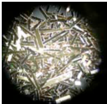
Figure 1. Photos of a) free-standing energetic multilayer foil (ruler is 15 cm long) and b) a coarse powder of energetic multilayer (particle widths \sim 400 \mu\text{M} ).
