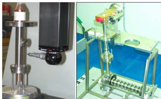
Fig. 1. Cold End Assembly on CMM and coupling test of the input coupler.
