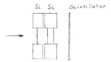
The first counter is a 200  $\mu$  surface barrier, totally depleted Li detector. The second is a 5 mm Si lithium drifted detector. A scintillation counter is behind the entire hodoscope. Very low energy protons are detected by the first element only.
