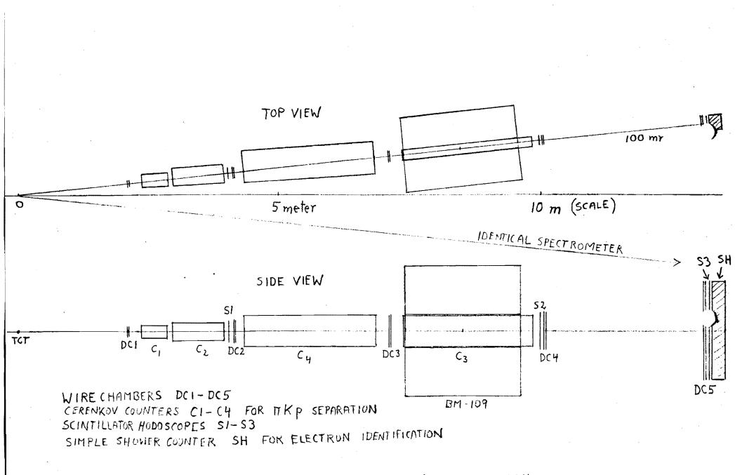
FIG 2 APPARATUS FOR HEAVY PARTICLE SEARCH
