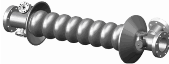
Figure 1: A naked third harmonic superconducting cavity.
