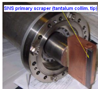
Figure 6: Spallation Neutron Source (SNS) collimator
