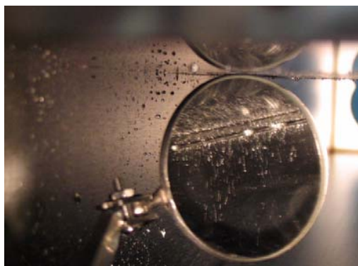
Figure 8: Collimator accident condition following beam miss steering at the FNAL Tevatron
