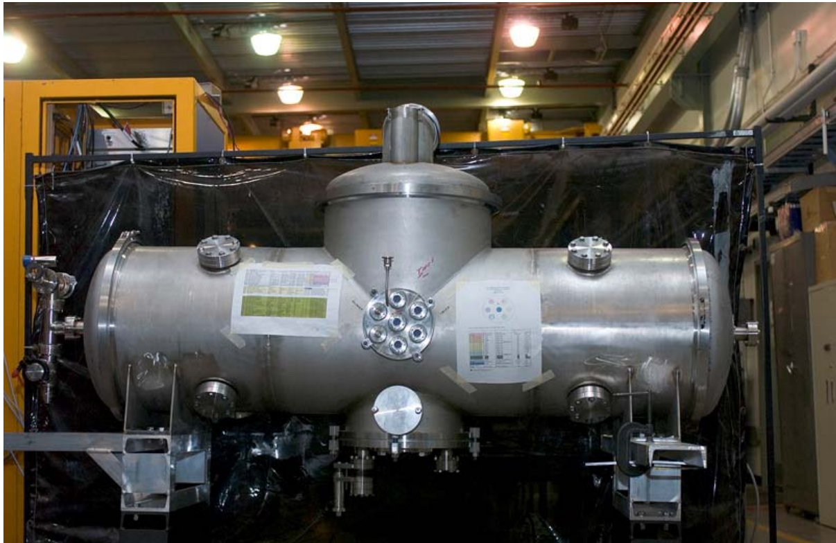
FIGURE 3. The CKM Cryomodule with 13-cell 3.9 GHz superconducting RF cavity
