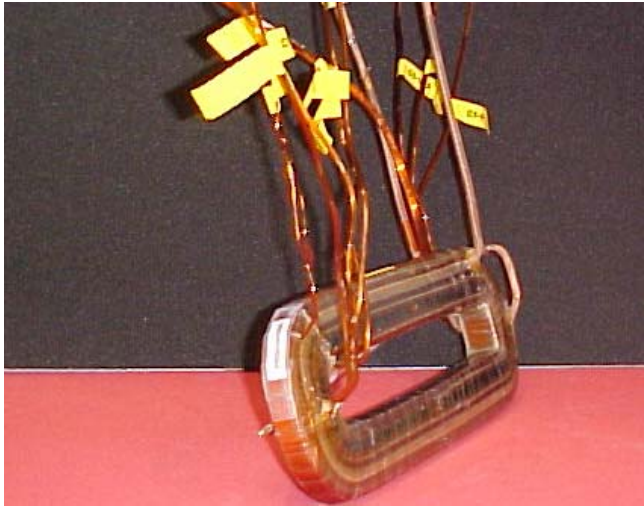
Fig. 4. Type #1 coil assembly appearance after the potting.
