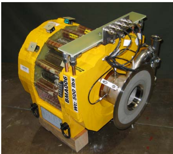
b) After coil leads were cut and connected...
