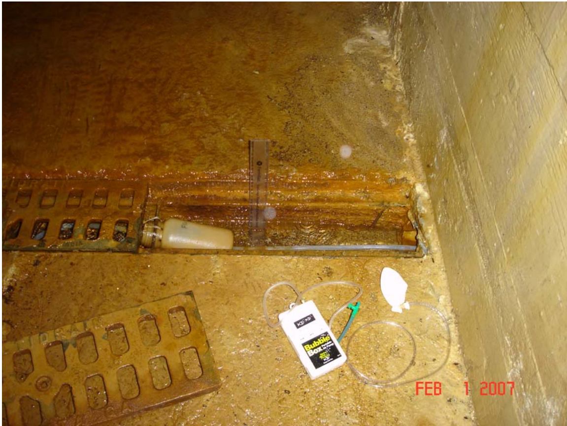
Figure B1. At Grate 1, the tube permanently installed for sampling the Main Drain is visible (but irrelevant). In the foreground is the air bladder for blocking the drain pipe in order to measure how fast the gutter fills up, and thus deriving the water flow rate.
