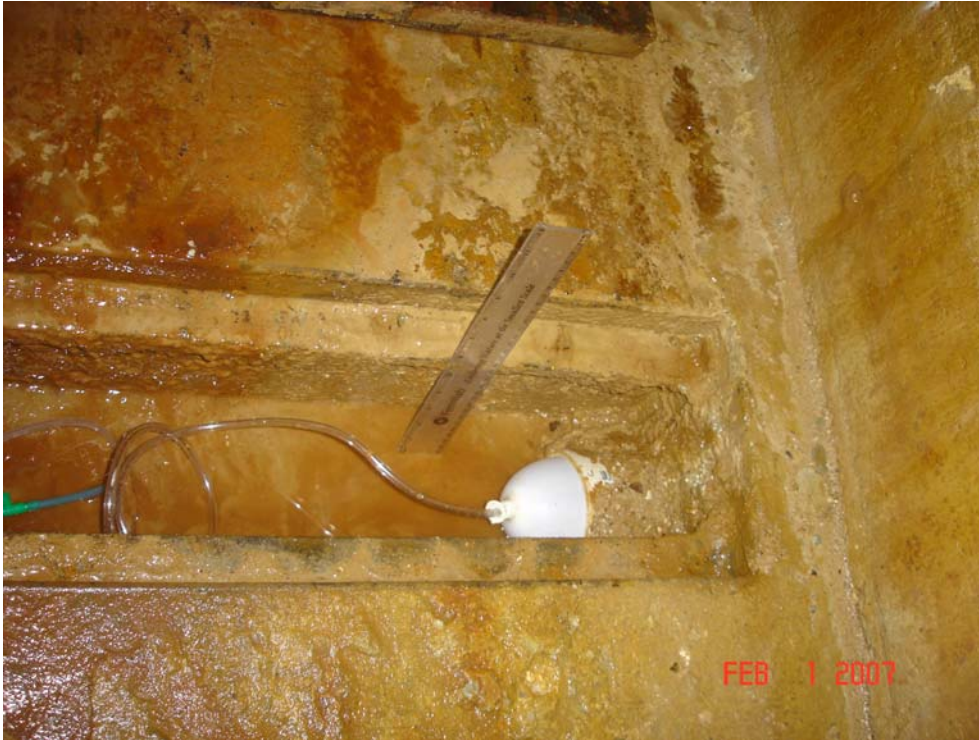
Figure B2. Air bladder blocking drain, and ruler for measuring increase in water height.
