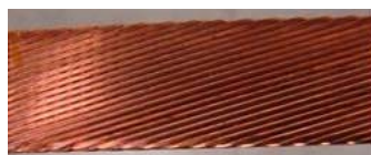
FIGURE 1. NbTi cable used for the insulation tests. It is 15.4mm wide identical to the cable used for the inner coils of the LHC interaction region quadrupoles.
