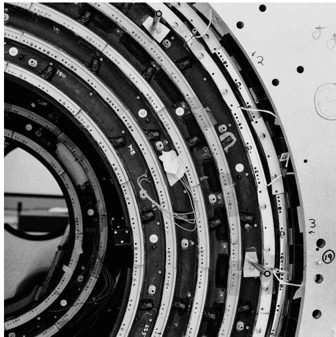
Figure 3.5: The fiber tracker detector, shown from the direction of the beam pipe.
