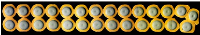
Fig. 2. Cross-section of rectangular Nb 3 Al Rutherford cable with low compaction factor 82.5 %. The F1 strands were used. 14.2 mm x 2.0mm.
