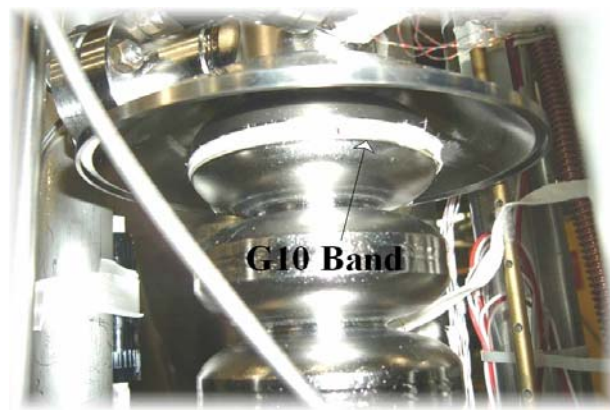
Figure 2: Cernox RTD thermometry G10 band wrapped around the cavity equator.
