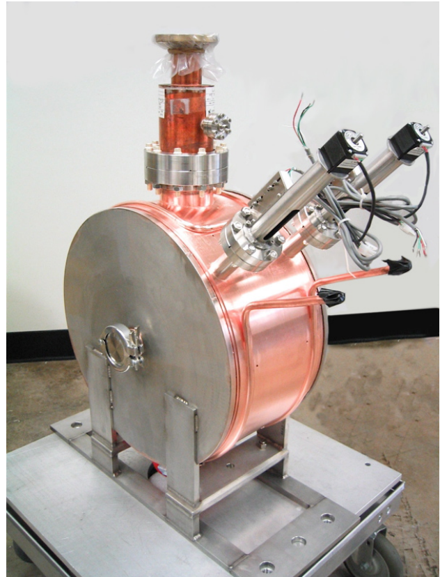
Fig. 3: The fully dressed prototype, the universal stand is visible at the bottom bolted to the resonator's support brackets. The same stand is used for all the resonators.
