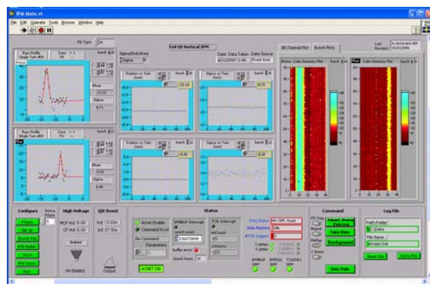
Figure 1. Screenshot from the Tevatron IPM Labview program. At low beta, the vertical system is capable measuring both protons and pbars simultaneously, without moving the detector.
