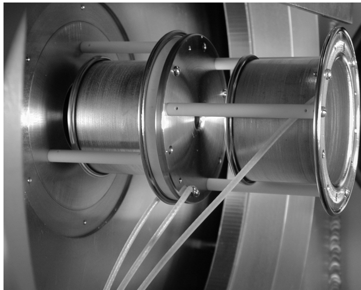
Figure 3-17: Photograph of the NTX beam scraper system.
