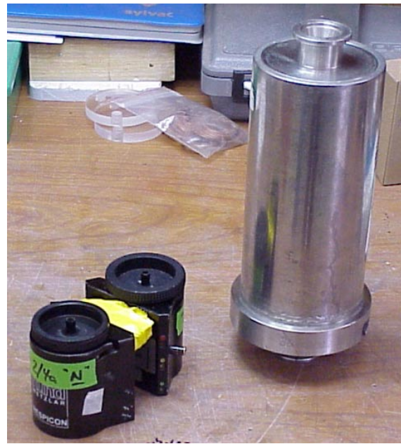
Figure 8. Aerosol Particle Samplers: Respicon Virtual Impactors (left) Berner Particle Impactor (right)
