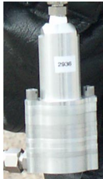
Figure 10. Marple Cascade Impactor 8-stages, 0.4 – 21 μm AED
