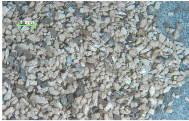
Figure 19b. Test 2/1B Impact Debris, 0.25 mm sieve
