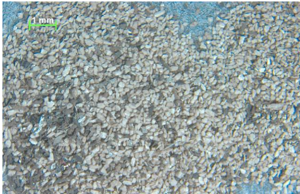
Figure 19c. Test 2/1B Impact Debris, 0.125 mm sieve
