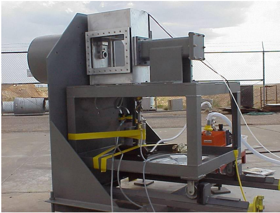
Figure 2. Phase 2 Surrogate – HEDD Impact Aerosol Test Setup, 2/4A & 2/4B, at Sandia ECF Gun Site
