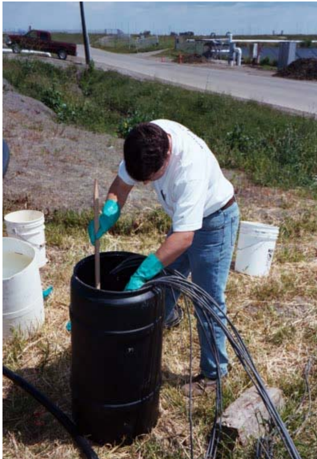
Image 47. Pressure transducers were tested for accuracy by submerging the sensors in water at various depths.
