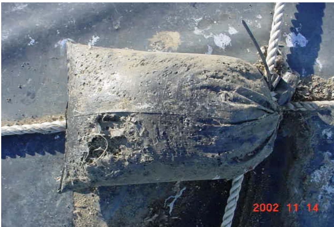
Image 48. Sandbag damaged by seagulls
