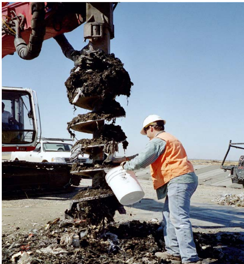
Image 38. At select locations, samples were collected directly from the auger to record the temperature of the waste as it was removed from the cell.
