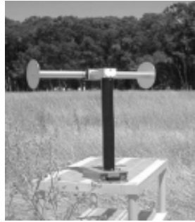
Figure 2.: HFI transmitting and receiving antennas: (a) Loop transmitter and related power supply; (b) Electric field sensor with a long supporting beam and a big base plate; (c) Magnetic field sensor.
