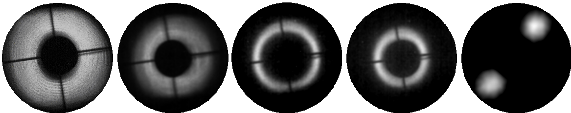
Fig. 2. EUV pupil fills recorded through the MET exposure system using the in-situ pupil-fill monitor. The illuminator can access a \sigma range of up to 1.2 in x and 0.8 in y .
