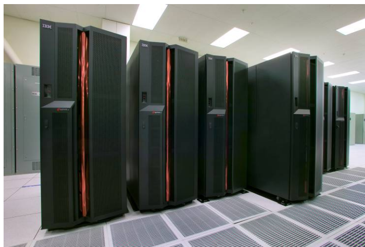
Figure 12. Bassi is an 888-processor IBM p575 POWER5 system with a theoretical peak performance of 6.7 teraflop/s.
