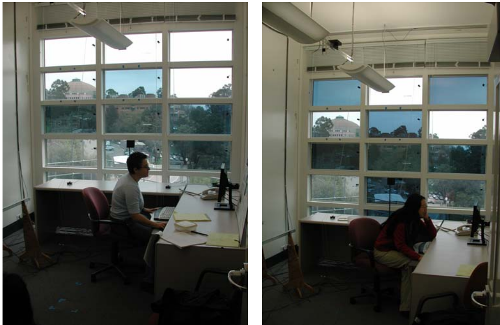
Figure 6. In a field test, occupants were provided with a web-based dimmer or slider switch so that they could manually switch individual EC windows to any transmittance level between fully clear and fully tinted. Occupants switched some EC windows for privacy, glare control, daylight, and view.
