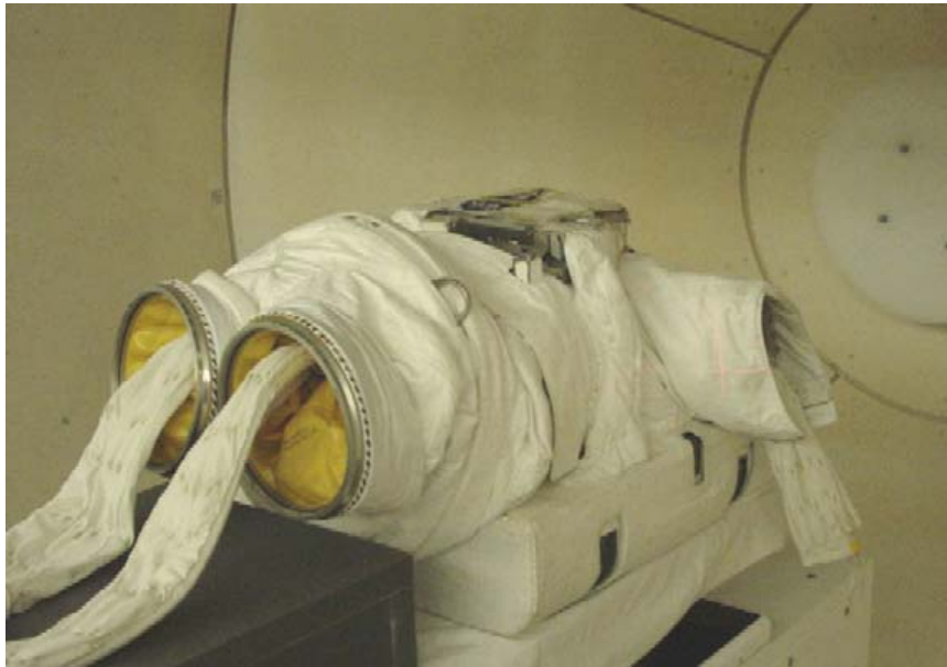
Figure 10. Torso portion of the EMU suit during exposure of stomach detector stack. The beam entered the suit from above.
