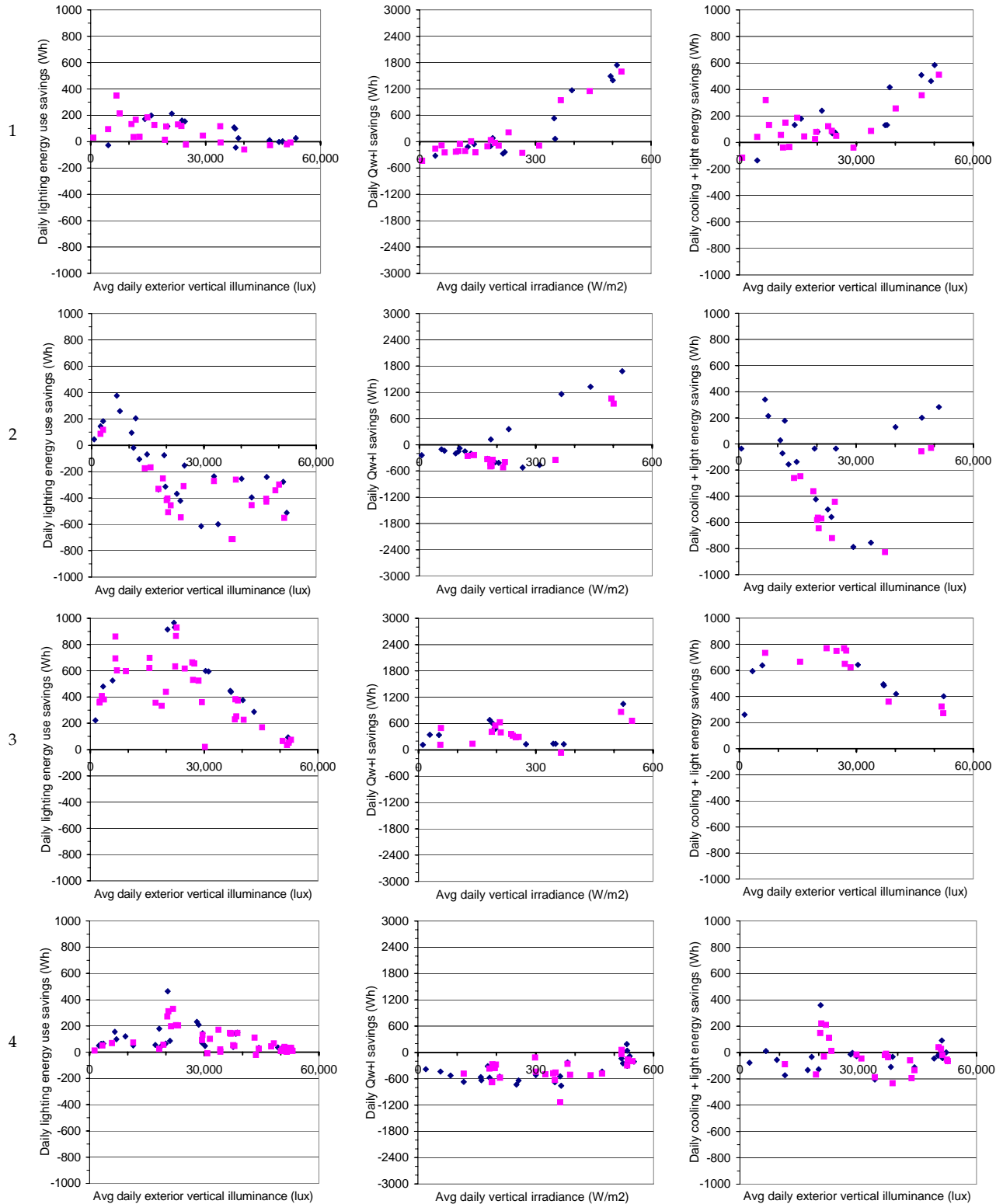
Figure 21. Average daily vertical illuminance or irradiance versus daily lighting energy savings (left), daily cooling load savings due to solar heat gains and lighting (middle), and net daily energy savings (right) for Cases 1 (top) through 4 (bottom). diamonds: Room B; pink squares: Room C.
