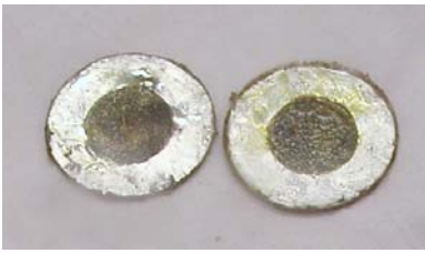
Figure 8. The presence of lithium coins after 10 cycles passing \pm 0.1 \text{ mA cm}^2 current in a (\text{Li} \mid \text{BMIMBF}_4 + 1 \text{ mol/kg LiBF}_4 \mid \text{Li}) cell. Shiny lithium metal on the outer layer and mossy lithium in the middle are clearly observed.
