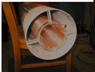
Fig. 5 Low voltage air dielectric model. The helical line on the left was driven directly by a voltage source connected to the input tap, while the
