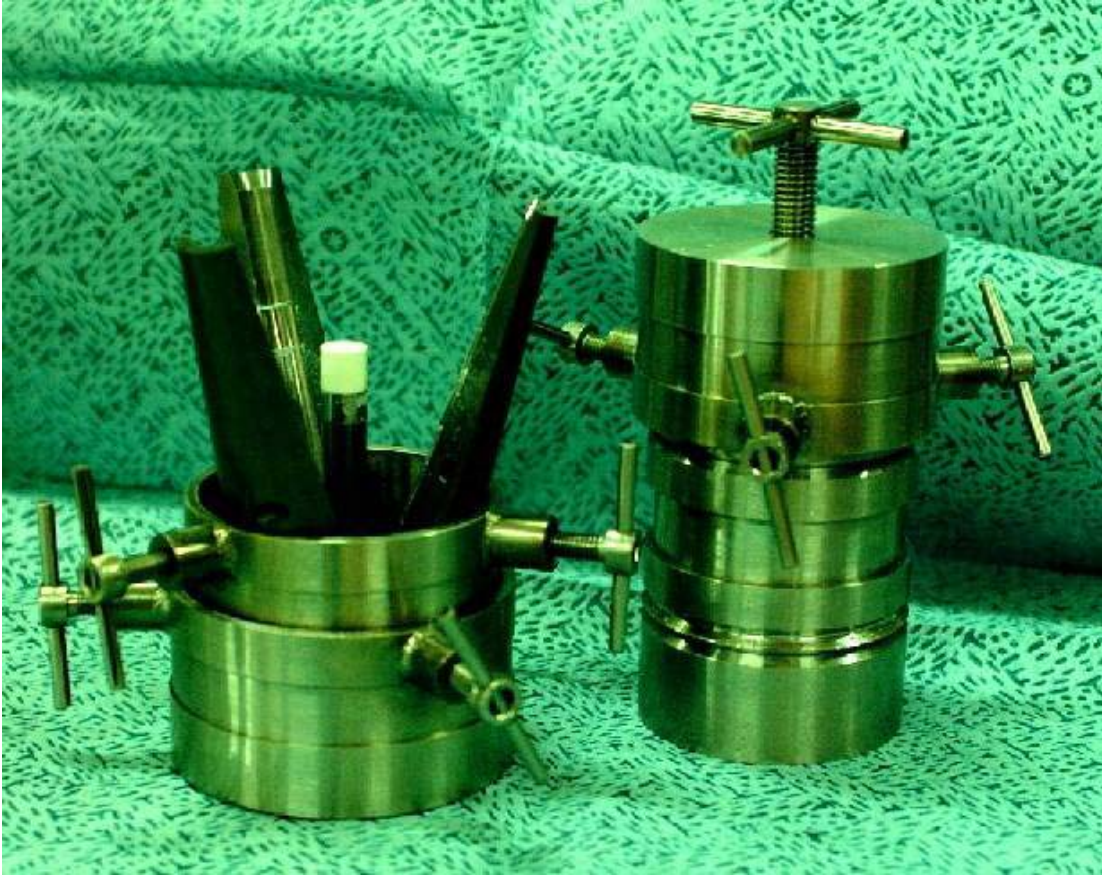
Figure 5: New tri-part press with for hot cell with MgO 2 pellet sample
