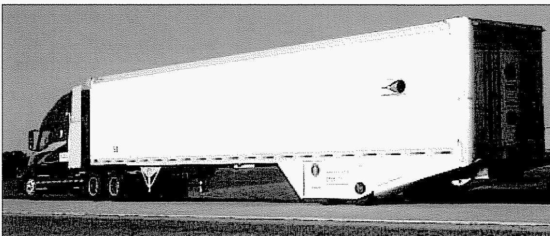
Figure 1- Modified Trailer during on-track SAE Fuel Economy Test II
