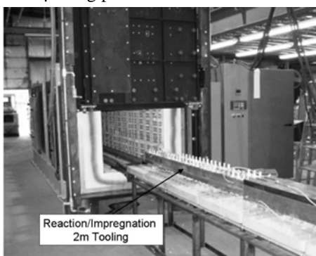
Fig. 6. Reaction/Impregnation 2 m tooling & 6 m furnace qualification.
