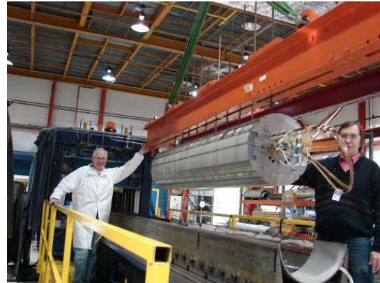
Fig. 6. HFD01 yoked mirror magnet being placed into the lower shell on the insertion table of the weld press.
