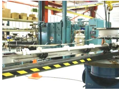
Fig. 3. LM02, 4 m RRP inner coil being wound with spool of outer cable suspended above the winding table.
