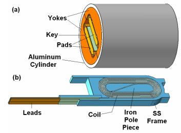
Fig. 1. Geometry of SR magnets.
