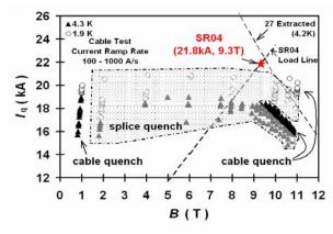
Fig. 9. The load line for SR04 magnet and its highest quench value 21.8 kA at 9.3 Tesla at 3.95 K are shown. Quench values of the F1 Nb<sub>3</sub>Al Rutherford cable tested at CERN at 1.9 K and 4.3 K are shown together.
