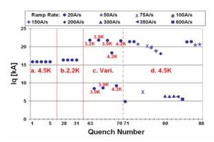
Figure 6. Quench history a) 4.5K 20A/s training with big ripples in current. b) 2.2K 20A/s training with big ripples, c) temperature dependence with reduced ripples, d) 4.5K ramp rate dependence with reduced ripples.
