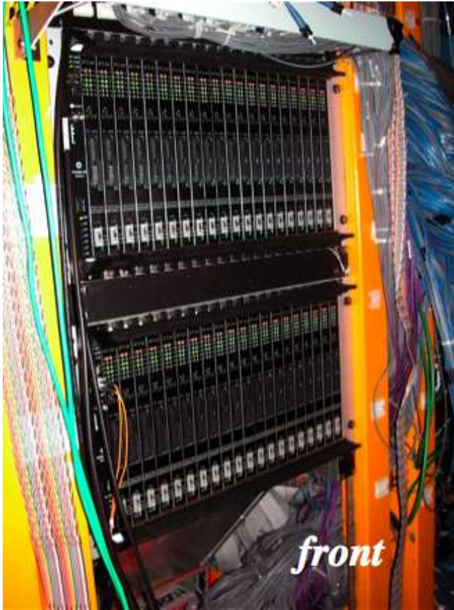
Fig. 3. The new track finding hardware installed under the D\emptyset detector. The 40 new DFEA2 boards are arranged in 2 crates, easily accessible from the front. The 320 input and 320 output cables are located in the back of the crates.
