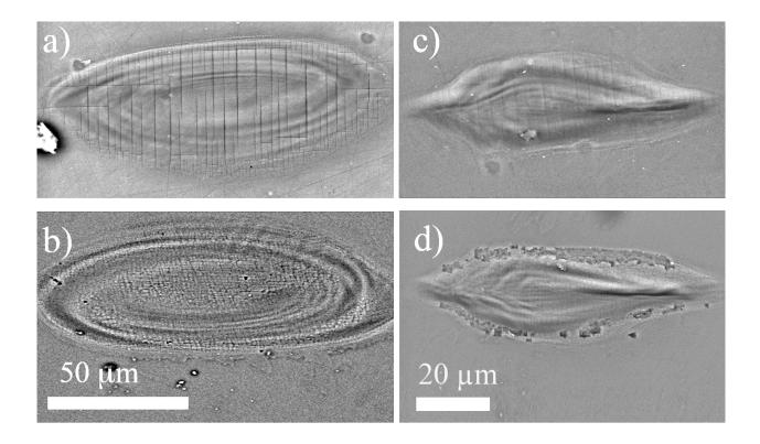
Fig. 3. SEM images of the ablated spots. The pictures a) and c) are obtained on LiF with 25 shots at the fluence of 0.8 and 3 J/cm<sup>2</sup>. Pictures b) and d) are obtained at the same fluences as a) and c) respectively, on  $CaF_2$  crystals.
