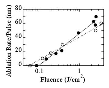
Fig. 2. Experimental ablation rates/pulse versus the fluence of the 46.9 nm laser for LiF (full circles) and  $CaF_2$  (empty circles). The solid and the dot ted lines are the results of the theoretical fittings obtained using the logarithmic curve (see formula within the text) for the two materials, respectively.
