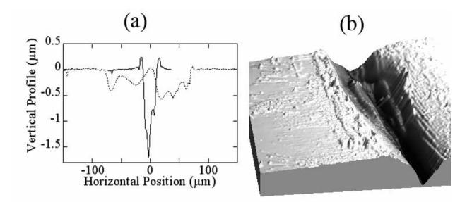
Fig. 1. (a) Experimental vertical profiles of craters produced on  $CaF_2$  by the 46.9 nm laser at the fluences of 0.36 (dotted line) and 3 J/cm<sup>2</sup> (solid line) using 25 laser shots. (b) AFM image of the crater produced on  $CaF_2$  with the f luence of 3 J/cm<sup>2</sup>.
