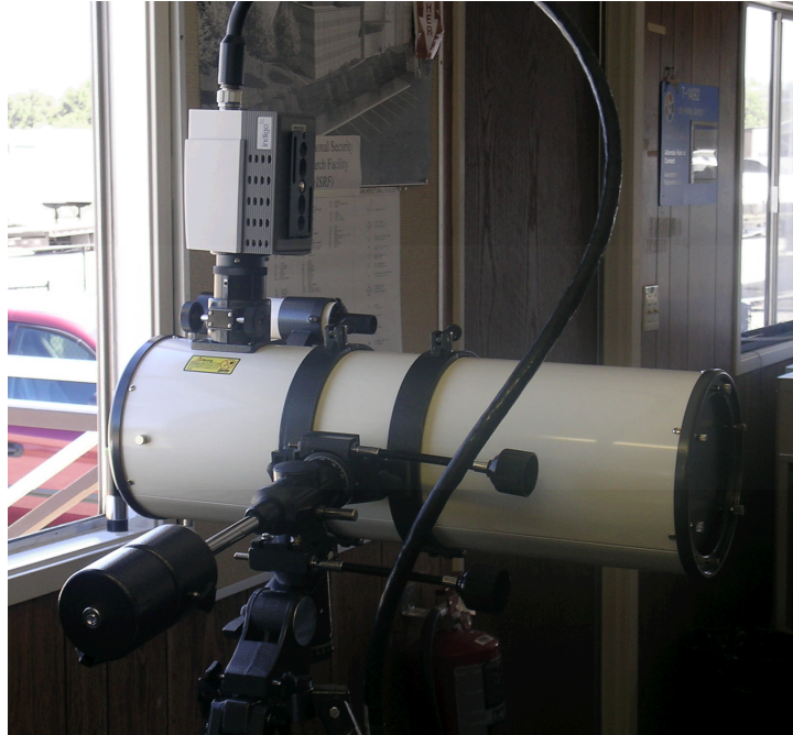
Figure 7: Newtonian reflector telescope with Indigo camera attached and looking out the (open) window of our observation location.
