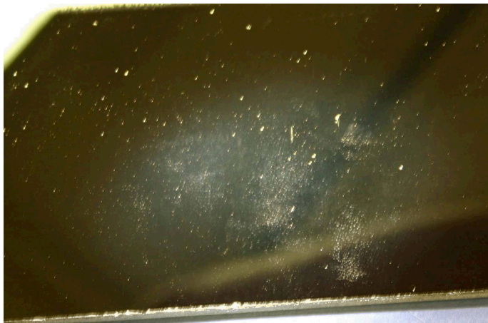
Figure 19. Smudges and particles on black glass caused by tapping and rubbing with a "clean room" glove that was not as clean as desired.
