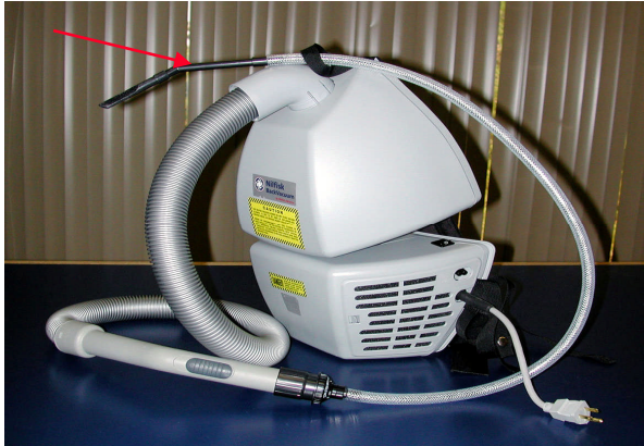
Figure 12. Nilfisk clean room backpack vacuum (“back vacuum”) with mini attachment for tight spaces.
