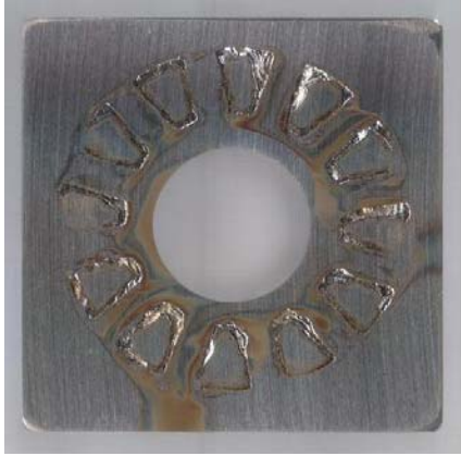
a) Side 1: Corroded surface under the PTFE-wrapped ceramic washer
