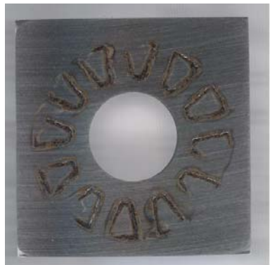
b) Side 2: Corroded surface under the PTFE-wrapped ceramic washer
