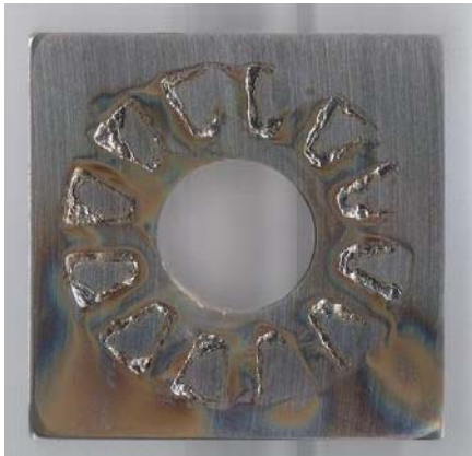
b) Side 2: Corroded surface under the PTFE-wrapped ceramic washer
