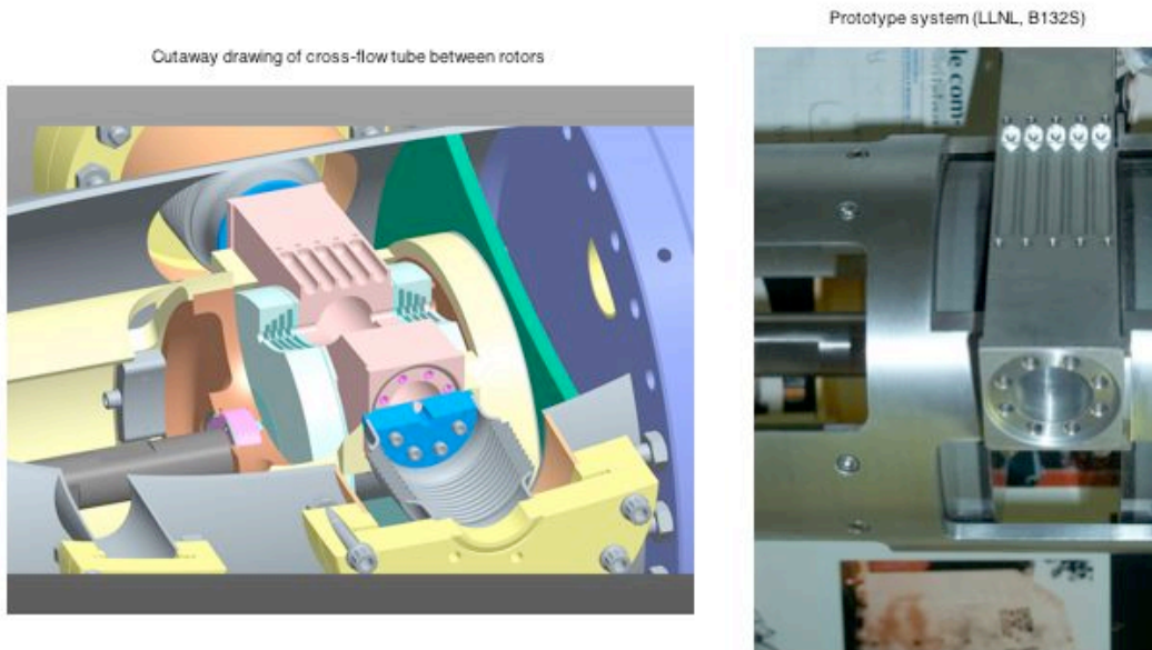
Figure 9: Cutaway drawing and photograph of cross-flow region in endstation flanked by baffled rotors. One of the primary goals in designing and fabricating these initial test units was to verify that we could achieve a gap spacing of \leq 0.002 " between these components. Note that the venturi that would normally be used in a production-line endstation was replaced by a rectangular cross-flow tube with a straight throat in this particular unit for use in tests with static gas.
