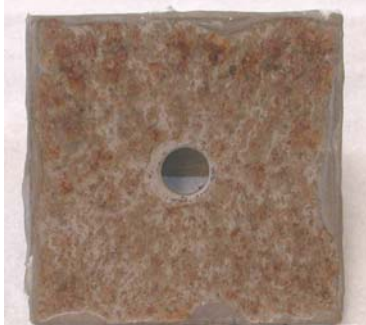
Original SAM40 (DAR40) – Corrosion After 13 Cycles
