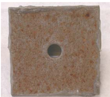
Type 316L Coating After Exposure for 13 Cycles
